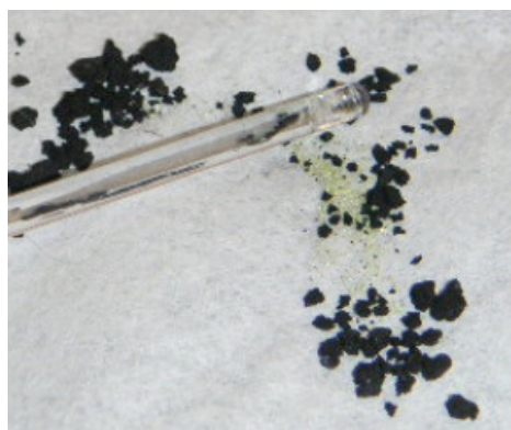
Fig. 1. Sulfur (light particles) removed from pore system of the sludge-derived adsorbent (black particles) via heating at 100 °C in vacuum.
