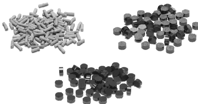
Fig. 2 Commercial HDS catalysts and sorbents (INS) a) hydrodesulfurization catalyst (HDS), b) zinc-copper sorbent Cu/ZnO, c) zinc sorbent ZnO.
