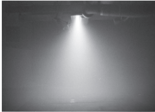
Fig. 1. The visible light glow indicates that the cold plasma is formed inside the process vessel in which gas is irradiated.
