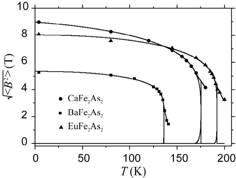
Fig. 9. Plot of square root from the mean squared amplitude of SDW  $\sqrt{\langle B^2 \rangle}$  versus temperature. Solid lines represent total, coherent, and incoherent contributions.
