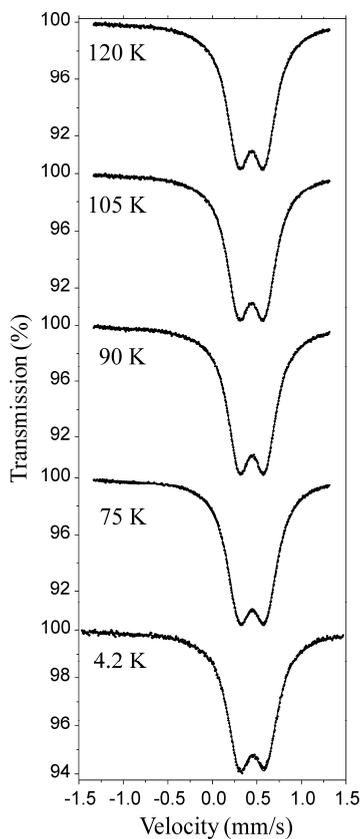
Fig. 4. Mössbauer spectra versus temperature obtained in the null external magnetic field. Spectra were collected for the low velocity range.
