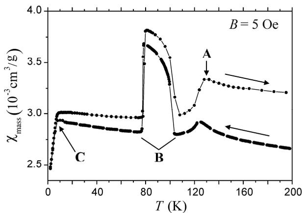
Fig. 3. Magnetic susceptibility measured versus temperature  $T$  upon cooling and subsequent warming of the sample. Applied field  $B$  is well below the first critical field.
