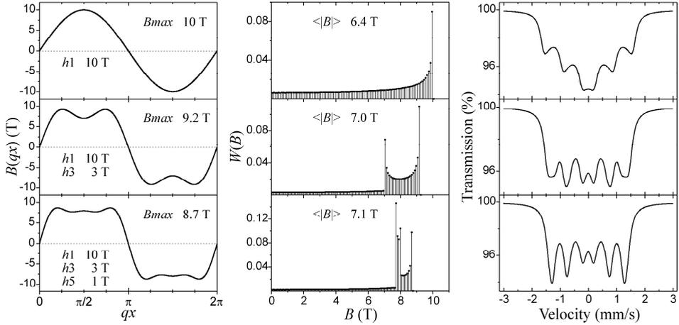
Fig. 2. Evolution of the SDW-shape, corresponding magnetic field distribution and shape of the Mössbauer spectra is shown versus addition of subsequent harmonics. The symbol  $qx$  stands for the phase of SDW,  $W(B)$  denotes field distribution function plotted versus the field  $B$ . Maximum amplitudes of SDW  $B_{max}$  and amplitudes of the harmonics  $h_n$  ( $n=1,3,5$ ) are shown as well. The symbol  $\langle |B| \rangle$  denotes average of the respective distribution.
