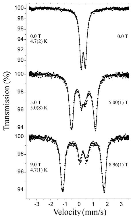
Finally, the spectra obtained in the strong external magnetic field oriented along the radiation beam are shown in Fig. 6. A standard  $^{57}\text{Co}(\text{Rh})$  source was kept out of the field and at the sample temperature (for all measurements without external field the source is kept at room temperature). Note that the field acting on the iron nucleus is practically an applied field despite low temperature
