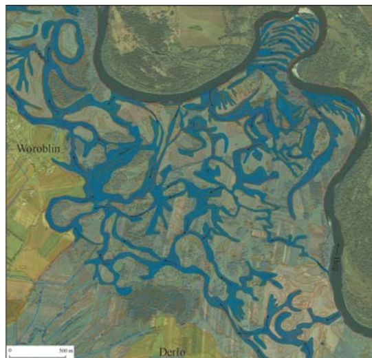
Fig. 6. The two-year floods in the left-bank Bug River valley, wide section of valley near Derło and Woroblin (based on Plan operacyjny ochrony przed powodzią... , 2003 and author's observation). Arrows mark the direction of flooding water in topographic depressions
