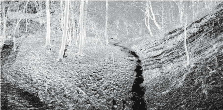
Fig. 3. Laser scanning scene (point cloud) with vegetation (before its removal from DTM)
